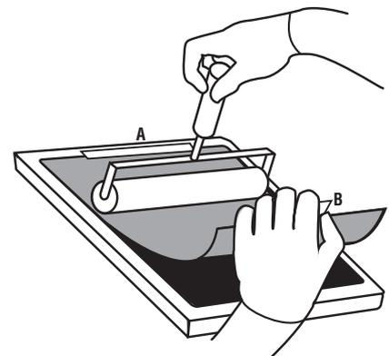
Relax film slightly allowing tab 'A' edge to come close to LCD panel, but not touch. With free hand, use roller to laminate film into place in one continuous sweep. Remove tabs 'A' and 'B'. Use plastic stylus to complete lamination along edges as necessary. Clean with acetone as necessary.
