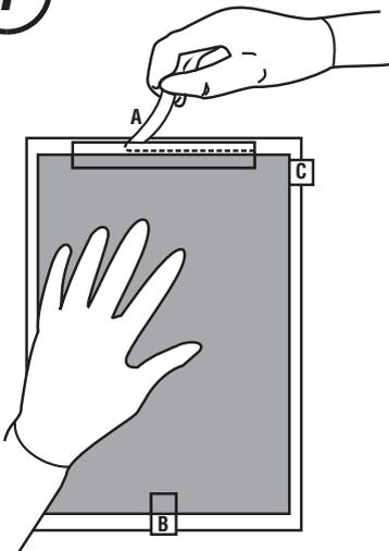
Place film, liner side down, onto LCD panel, and center within metal bezel. Holding film firmly in place with one hand, remove liner from tab 'A' and adhere tab A to metal bezel. Check film alignment; realign if necessary. Then place tab 'B', Scotch® Brand Tape on the top surface of the film.
