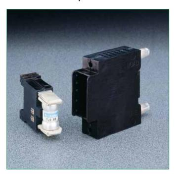
Littelfuse compact LTFD 101 fuseholders for TLS fuses are designed for quick installation into telecom equipment panels. Their modular design fits into spaces originally designed for circuit breakers and they can be front panel mounted or rear mounted using bullet connectors. The innovative new pull-out design eliminates the need for tools to replace fuses and includes an alarm signaling circuit to identify the blown fuse.
