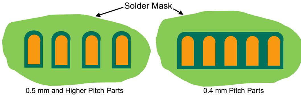
For the cases where the thermal land dimensions are close to the theoretical maximum discussed above, it is recommended that the thermal pad area should be solder mask defined in order to avoid any solder bridging between the thermal pad and the perimeter pads. The mask opening should be 100 microns smaller than the thermal land size on all four sides. This will guarantee a 25 micron solder mask overlap even for the worse case misregistration.
