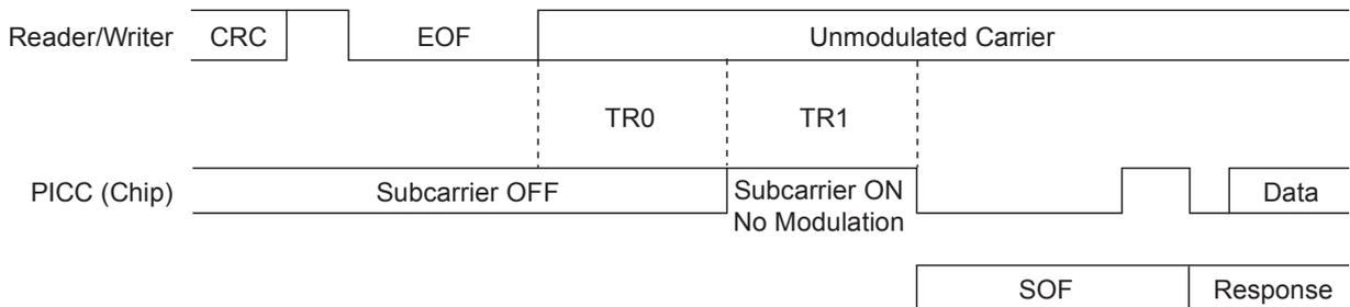
The FWT is the maximum time that a PICC requires to begin a response. The PICC transmits a parameter in the ATQB response to the polling command that tells the reader the worst case FWT. The PCD is not permitted to modulate the RF field while waiting for a PICC to respond to a command. Modulation of the RF field during a PICC memory read or write operation may corrupt the operation or cause reset of the PICC.
