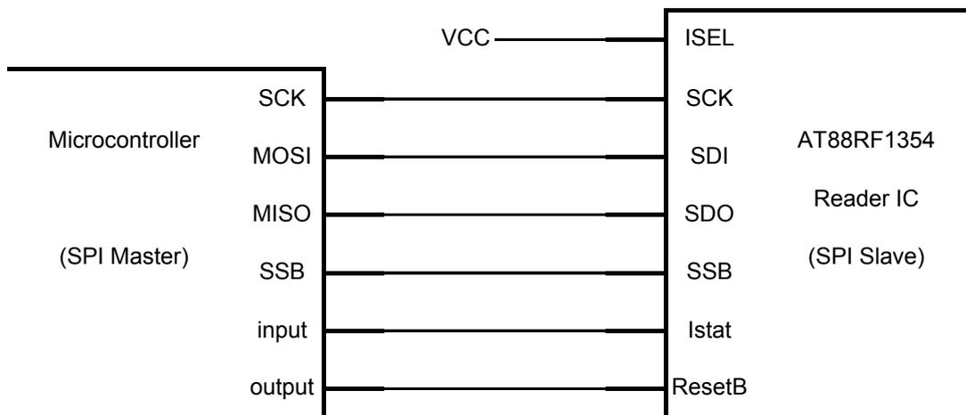
A high level on the ISTAT pin signals the host microcontroller that a byte of data is ready to be read from the AT88RF1354 serial interface. If another byte is immediately available on the serial port, ISTAT will go low for 150 uS, then return high. ISTAT will remain high until the last bit of the byte is read, when it will return low. All data must be clocked out of the AT88RF1354 before it can receive a command.
