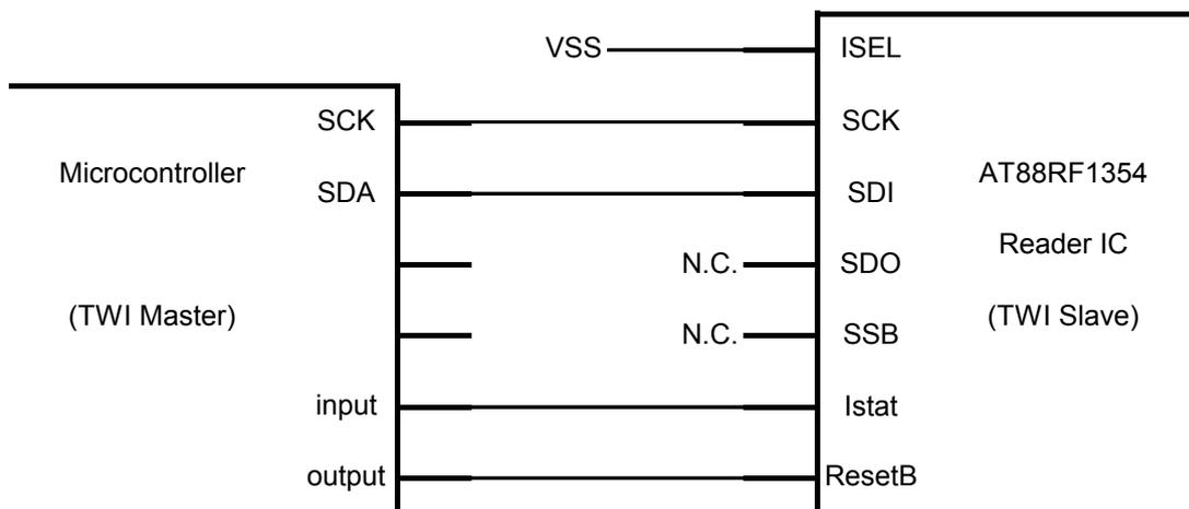
A high level on the ISTAT pin signals the host microcontroller that a byte of data is ready to be read from the AT88RF1354 serial interface. If another byte is immediately available on the serial port, ISTAT will go low for 150  $\mu$ S, then return high. ISTAT will remain high until the last bit of the byte is read, when it will return low.
