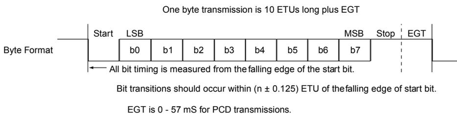
Despite the fact that data transmissions occur LSB first, all of the commands, data, and CRC bytes in ISO/IEC 14443 and in this specification are listed in the conventional manner, with MSB on the left and LSB on the right.
