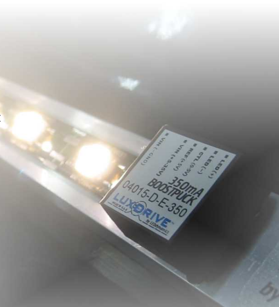
4015 BoostPuck LED Driver Module powering (9) LEDs in series at 350mA ( V_m=12V )
