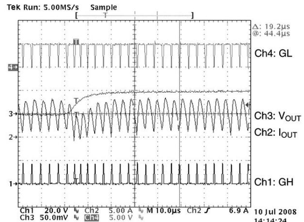
Transient Response:  $V_{IN} = 12 V$ ,  $V_{OUT} = 1.2 V$ ,
