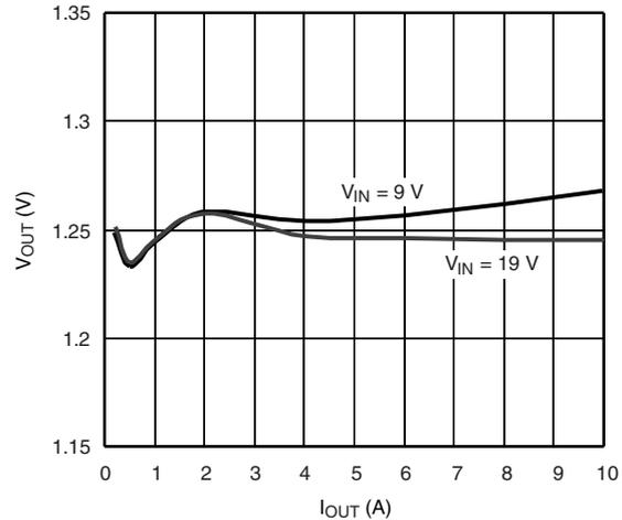
Load Regulation, ( $V_{OUT} = 1.2 V$ )
