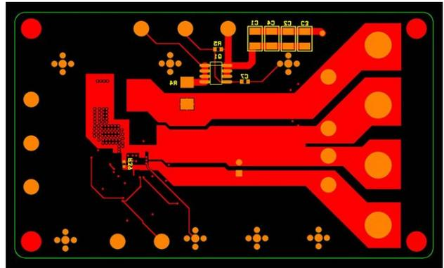
Figure 19. PCB Layout - Bottom Layer
