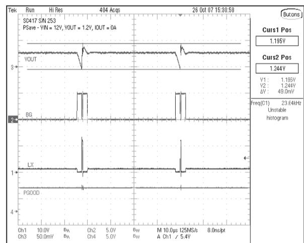
**Figure 6 - Ultrasonic Power-Save Operation Mode**
