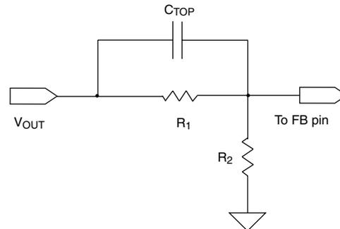
Figure 13 - Capacitor Coupling to FB Pin
