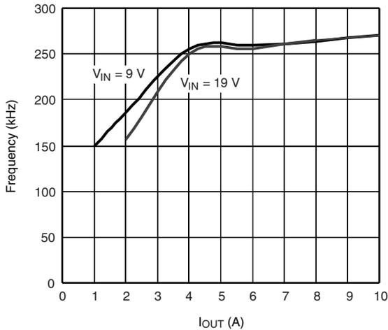
Frequency vs.  $I_{OUT}$ , ( $V_{OUT} = 1.2 V$ )
