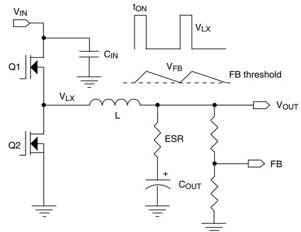
Figure 1 - Output Ripple and PWM Control Method
